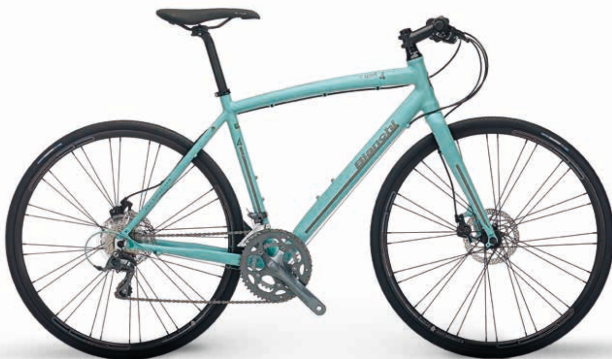
CAMALEONTE C-SPORT 4 ALU CLARIS 2X8SP COMPACT DISC BRAKE AND CARBON FORK 28MM TIRE
