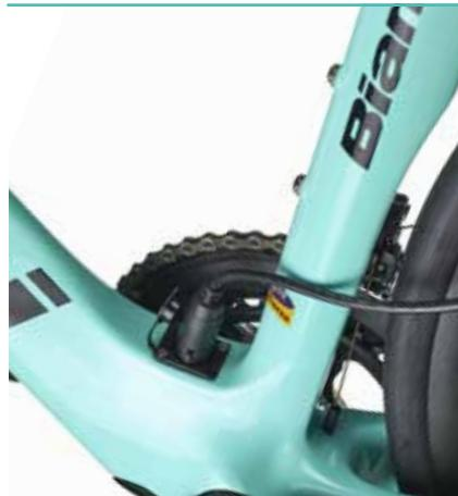
The X35 V.2 M1 motor is powered by a slim, 40mm wide 250W battery, positioned inside the downtube of the Aria e-Road frame.
