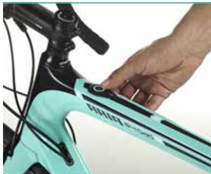
Bianchi engineers integrated the iWOC One flush-fit power and battery level controls unobtrusively into the Aria e-Road's aero top tube.
