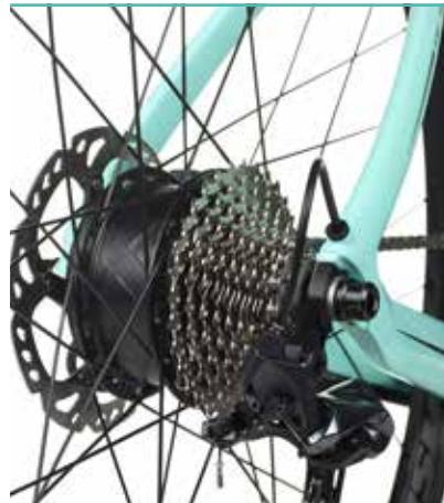
Nestled between the rear cassette sprockets and the rear disc brake rotor, the motor is virtually hidden.
